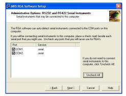
The RGA software continuously attempts to connect to an RGA instrument on all of your computer's serial ports unless you identify particular ports as being 'RGA-disabled'.
