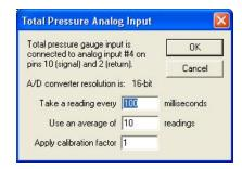
The Properties button shows a dialog in which you can change the acquisition frequency/accuracy. The software automatically converts the voltage to a pressure according to the manufacturer's
