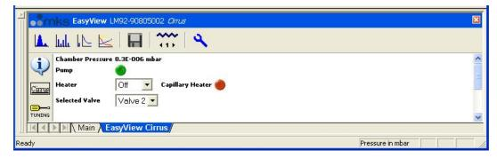
The chamber pressure is the value obtained from the internal gauge situated close to the turbo pump. Click on an indicator to change its state. If you have a multi-valve inlet you can change the active inlet using the drop-down list. The list always shows the currently active inlet.
