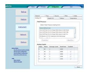
This tab displays the configuration of the Analog I/O connector on the rear panel of the control unit.
