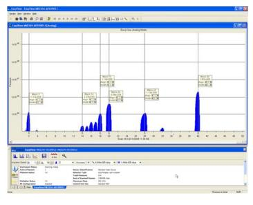
While in the mass tuning mode mass alignment flags are placed on screen. The vertical position of these flags can be adjusted if needed.
