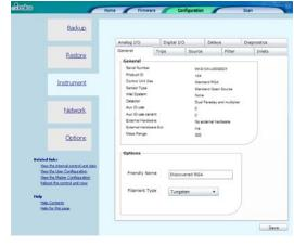
The General tab displays many fixed items of information, including the embedded software versions. The three user-configurable settings are the name assigned to the control unit, the mains frequency and the filament type. You may also use this page as another way to download new embedded software to the control unit.
