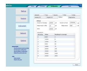
This tab is an advanced feature. The control unit has a table of software delays that control the length of transition states – for example how long to wait when switching between a Faraday and multiplier detector.
