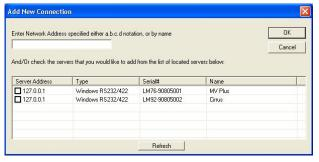
The list shows all the servers that are on the network and all the serial instruments connected to this computer (on 127.0.0.1).
