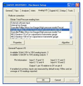
If, as in the example shown, the control unit is one with a pressure gauge attached, select the type of gauge from the list in the top panel.
