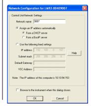
You have a basic choice between assigning a fixed IP address and having a computer on the network assign one for you. This latter case is called DHCP addressing, but please ensure that you only select this option if you have a DHCP server on the same network as the instrument.
