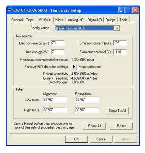
In the example shown the settings relate to the Base Pressure RGA configuration in which the electron emission current is 0.39mA and the ion energy is 7eV.
