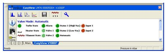
You have full control over the RVC settings using this panel. You can start and stop the pump, select the valve mode or open or close individual valves. Remember that, in order to open valves, the pump must be at speed and the RGA filament must be on.
