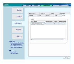
This tab will only be relevant if you have an RGA with an inlet system. Where this is the case you must configure each inlet so that its inlet factor (pressure reduction factor) is correct. If you obtained the complete system from MKS, you will have been informed what the inlet factors for your system are.
