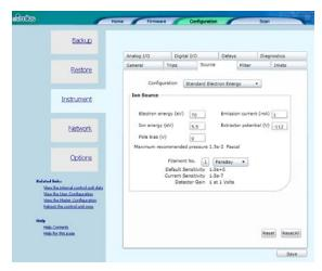
This tab shows the ion source and mass filter configuration properties for each of six possible groups of settings. You select the information displayed by choosing a **Configuration** from the drop down list at the top of the page.
