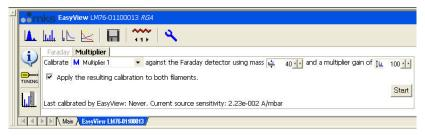
Select the multiplier setting to be calibrated from the drop down list, the mass to calibrate against and the multiplier gain required. By convention you typically calibrate Multiplier1 to have a gain between 30 and 100, Multiplier2 to have a gain between 100 and 1000 and Multiplier3 to have a gain greater than 1000. The multiplier will be calibrated at the mass chosen, so that the pressure reported in faraday and multiplier at this mass will be the same.
