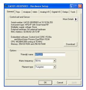
The General tab displays many fixed items of information, including the embedded sof tware versions. The three userconfigurable settings are the name assigned to the control unit, the mains frequency and the filament type. You may also use this page as another way to download new
