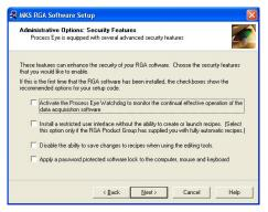
The **Watchdog** is a system tray application that continually checks that the main Process Eye application is running correctly. If it detects that it is not, it can shut it down and restart it.
