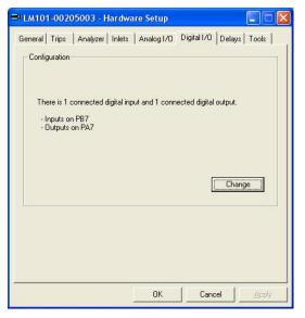
By default there are no I/O channels enabled but you can set individual channels to be configured as inputs or outputs by clicking the Change button.
