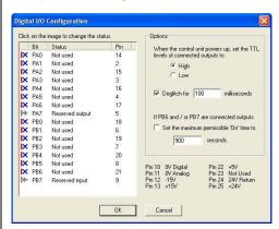
There are usually sixteen available channels of I/O, although if you have an external gauge on the analog input (as shown in this example), one or more channels may be marked as reserved.
