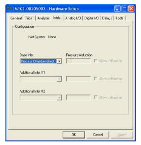
Select an item from the drop down list that describes as closely as possible the inlet that is fitted - for example a 'x10 orifice'.
