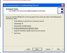
If you can do so, enter the instruments status by checking the LED's on the instruments rear panel and indicating the state of the LED's on this page.
