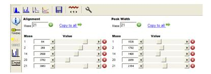
Entries for the alignment, width or both can be deleted using the red "X" icon.
