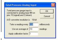
The **Properties** button shows a dialog in which you can change the acquisition frequency/accuracy. The software automatically converts the voltage to a pressure according to the manufacturer's calibration. You can change this calibration with a factor in v5.21 onwards. Values in excess of one increase the pressure relative to the manufacturer's calibration and values less than 1 reduce it.
