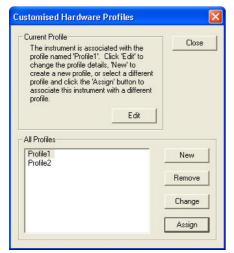
You can change the profile assigned to the current instrument by highlighting the profile in the list and clicking **Assign**.
