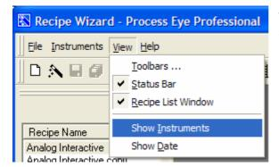
To show the instruments that each recipe is associated with select **Show Instruments** from the View pull down menu
