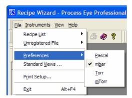
From the Recipe pull down menu select **Preferences** and then the units you wish to use. The currently available units are Pascal, mBar, Torr or mTorr. The units in Recipe Wizard do not have to be the same as those in Process Eye. However the setup applications can be used to set a common set of units throughout the whole application suite.
