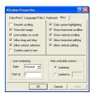
There are a number of miscellaneous properties that can be switched on or off by checking the boxes next to them. In addition format the line numbering by selecting the style of number to be used and the number of the first line. Change the number of actions that are store in memory so they can be undone by selecting **Limited to** and entering a number. By default the number of actions stored to be undone is unlimited.
