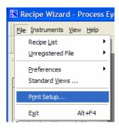
To set up the printer select **Print Setup** from the recipe pull down menu. This will bring up a standard windows printer setup dialog.
