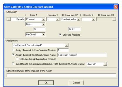
The Channel "Too Much Nitrogen" as defined above can be used to trigger the alarm when it becomes true.
