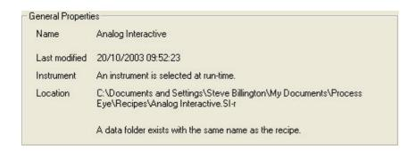
Included in general properties is the name of the recipe as it appears in the recipe list, the date the recipe was last modified, the name of the instrument associated with this recipe (in this case the recipe is generic and has no specific instrument associated with it) and the file name and location of the recipe file. If there is a folder in the data directory with the same name as the recipe this information will also be displayed.
