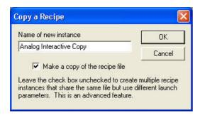
Enter the name of the new recipe; this is the name that will appear in the recipe list. By default there will also be a copy of the recipe file made with the same name as that entered into the text box but with a .SI-r extension.
