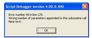
This is because the Msgbox function needs at least one parameter, the text to display
