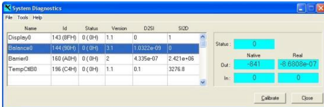
Image 4.15: The System Diagnostics and Calibration window used to calibrate devices.
