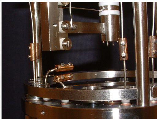
FIG. 8: Both wires removed and filament base is now isolated.
