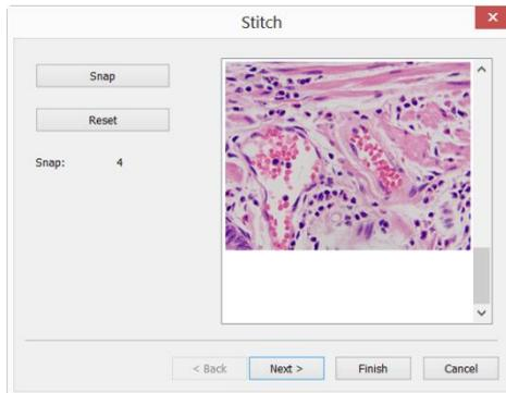
**Snap:** Click to capture image from camera. One should try to move the slide to a prop position to capture the desired images. In the moving process, the next image should have some overlaid area with the previous left or up image to ensure the
