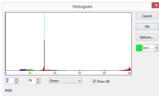
: [Left Value](#) in the currently selected region of histogram segmentation, corresponding to [Left Vertical Line](#) position in histogram. Users can segment the pixels bigger than the [Left value](#) by inputting a value in this edit box or dragging the [Left Vertical Line](#) in histogram. When input a [Left Value](#) in this edit box, users should
