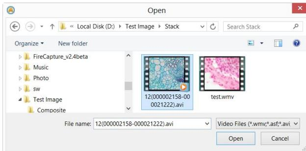
2. Select the name of the file you want to open. If the file does not appear, select the option for showing all files from the **Files of Type** combobox. The video file type can be **\*.wmv\***, **\*.asf\*** or **\*.avi\*** format.
