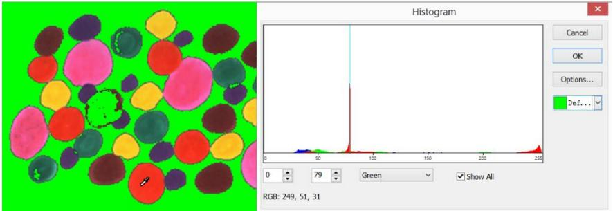
2. Move **Color Picker Cursor** to any pixel of the image, shown as above, **RGB** value of the current pixel will be displayed in the bottom Histogram window. Here **R** is 249, **G** is 51, **B** is 31, showing the **RGB** value of the ideal segmentation area, record the three values.
