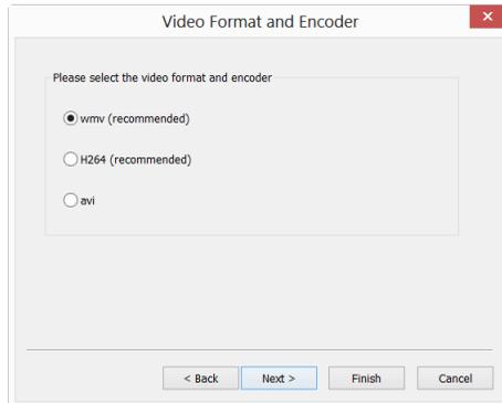
3. An **Encoder** dialog will be brought up. Here you can select the **Encoder** format, set the **Bitrat(Kbps)(256-16384)**, **Quality (1-100)** and **Key Frames Spacing (1-30)**. Click **Back** to return to the **Video Format** dialog, or **Next** to the next step;
