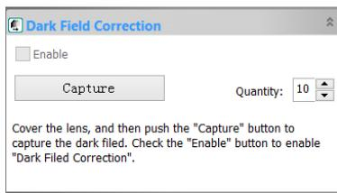
To [Enable](#) the [Dark Field Correction](#), one should capture the dark field image first. After the images are captured, the [Enable](#) button will be enabled. Check it will enable the [Dark Field correction](#). Uncheck is will disable the [Dark Field Correction](#).
