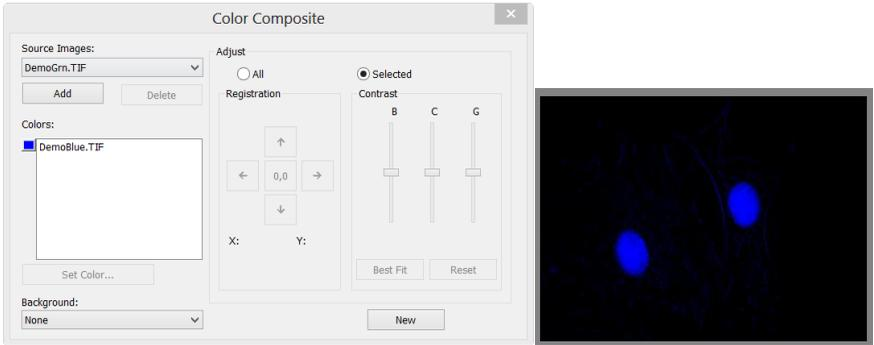
**Source Images:** The **Source Images** combo box displays the images available for color mixing. The **Source Image** list is initially filled with a list of the gray scale images that are currently open. The size of the color composite is determined by the first input image selected. Once this is entered, the list is filtered to contain only images of the same size as the initial selection.
