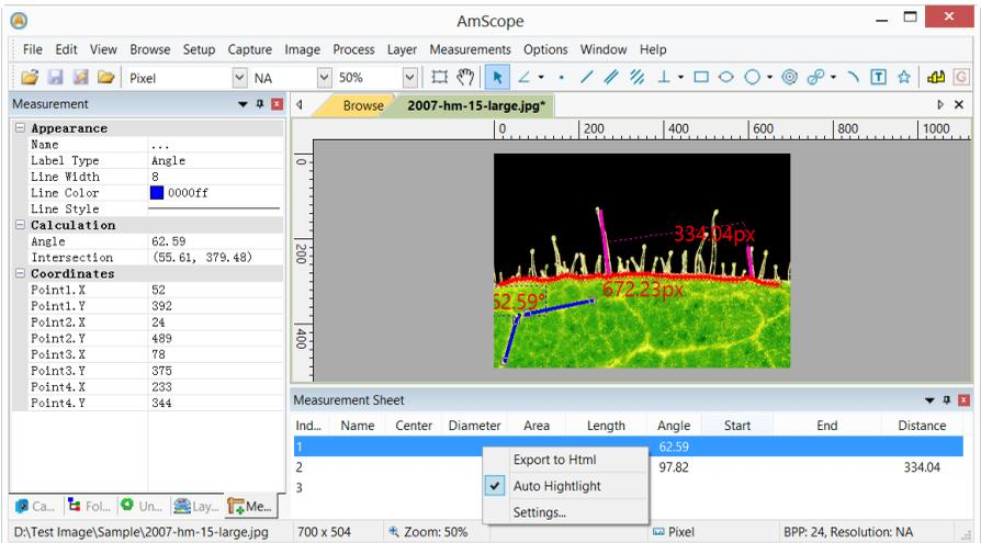
When choosing the [View>Measurement Sheet](#) command, the [Measurement Sheet](#) will be active. The [Measurement Sheet](#) shows the [Object's](#) possible features, such as [Name](#), [Center](#), [Radius](#), [Area](#), [Perimeter](#), [Angle](#), [Start Point](#), and [End Point](#) overlaid on
