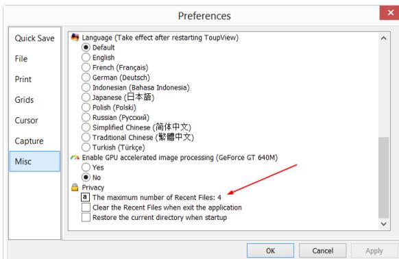
Here, clicking the **4** (default) edit box will allow you to enter the number of the **Recent Files** submenus that you want. The value ranges from **0** to **8**, the default is **4**; b) One can also check the **Clear the Recent Files when exit the application** to clear the **Recent Files** after exit AmScope application.
