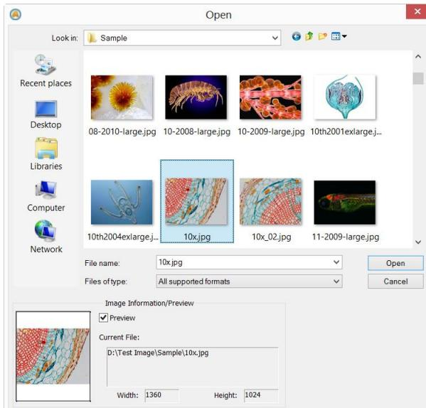
More than one image can be opened within AmScope simultaneously by a) with [Ctrl + left mouse button](#) method and b) [Shift + left mouse button](#) method to highlight the files to be opened. In this mode, the [Preview](#) window will be disabled.
