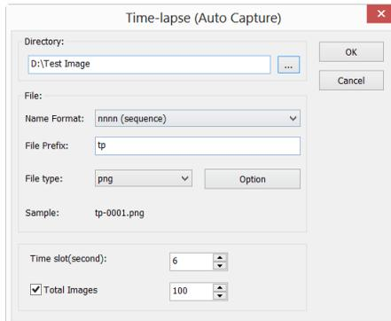
This function can capture a sequence of pictures with the specified time interval; you can precisely set the time interval (2 to 3600 seconds) and the total number of images(1 to 9999).
