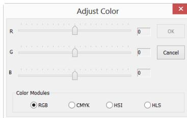
**RGB:** AmScope uses the **RGB** model. It assigns an intensity value to each pixel ranging from 0 (black) to 255 (white) for each of the **RGB** components in a color image.
