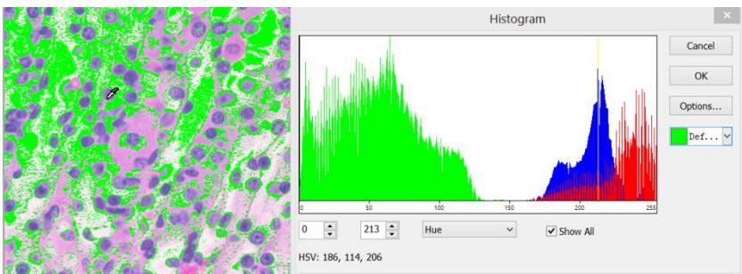
2. Move **Color Picker Cursor** to any pixel of the image, shown as above, **HSV** value of the current pixel will be displayed in the bottom Histogram window. Here **H** is 186, **S** is 114, **V** is 206, showing the **HSV** value of the ideal segmentation area, record the three values.
