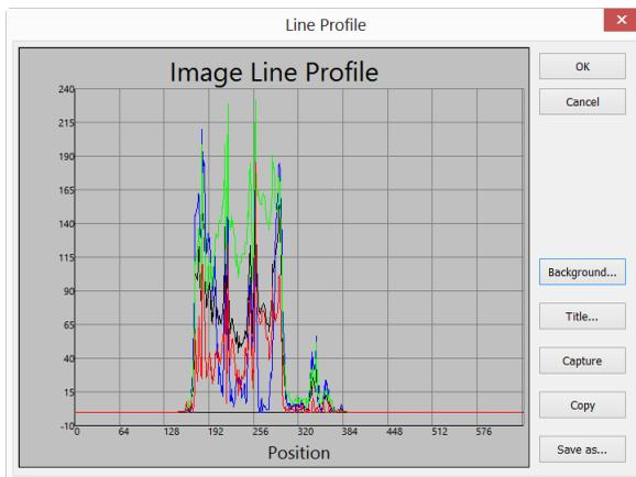
**Line Profile:** In a [Line Profile](#), the X-axis represents the spatial scale, and the Y-axis represents the intensity values which range from 0 to 255. If the image is a gray scale image, the gray value will be profiled. If the image is a HSV color image, the R,G and B values will be profiled separately with the corresponding R, G and B colors
