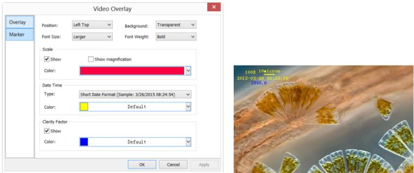
The **Position**, **Background**, **Font Size**, **Font Weight** of the **Scale**, **Magnification** and **Date Time**, and **Clarity Factor** can be defined together. Their **Colors** can be defined separately.
