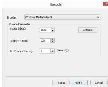
This dialog is used for the setup of video [Encoder](#) parameters for broadcasting. This setup dialog is just the same as those of [Capture>Start Record...](#) setup dialog. It mainly including [Encoder](#), [Encode Parameter](#) such as [Bitrate](#), [Quality\(1-100\)](#), [Key Frame Spacing](#) in second et al.
