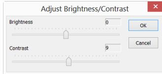
**Brightness:** Dragging the slider bar to the left decreases the level and dragging it to the right increases the level. The numbers on the right of the slider bar displays the **Brightness** value. Values can range from **-100** to **+100**. Default is 0;
