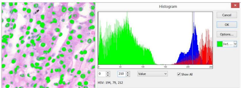
It's easily found that here S channel, defined 90~130, its lower limit is too big to get the pixel segmented. Then initial interval for S channel can be adjusted from 90~130 to 60~130 to segment the pixels nearby. (Note: If the background pixels of a single channel is within the initial interval, no segmentation change will take place. Only all
