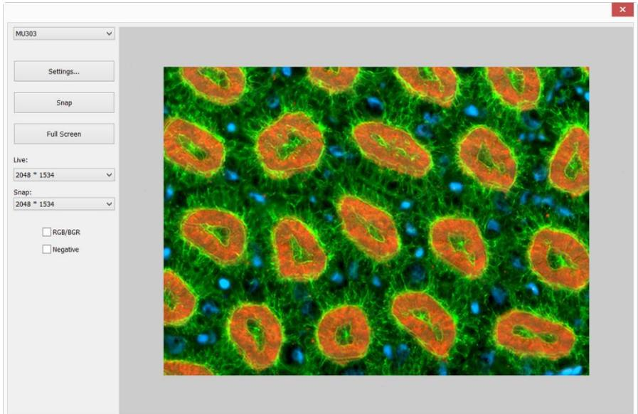
In this dialog, the video [Resolution](#) can be chosen. The [Video Source Property](#) can be set by clicking the [Setting...](#) button. Click the [Snap](#) button to capture an image. This will create a new window and its title bar will be assigned a digital as the image window name;
