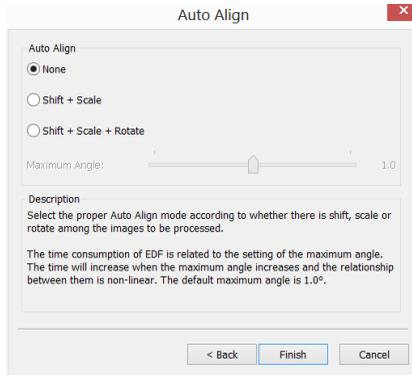
[None](#): Considering no [Shift+Scale+Rotate](#) among the selected images in the fusion process;
