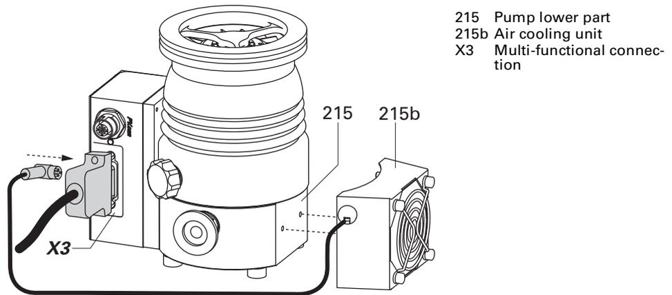
**Fig. 8: Connecting the air cooling unit**
