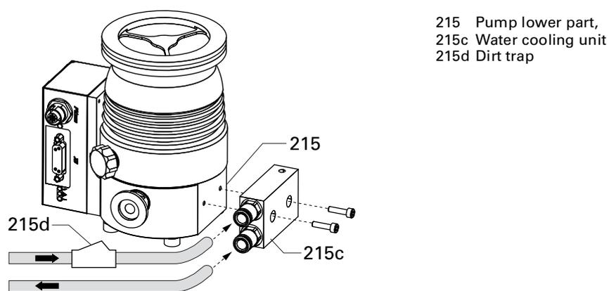
Fig. 13: Connecting the cooling water
