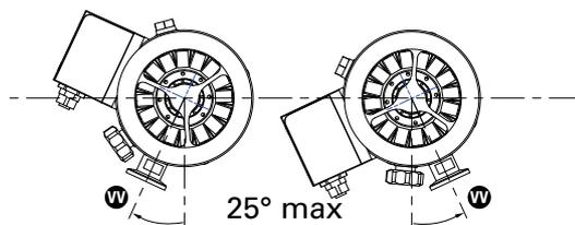
Fig. 4: Recommended orientation of the fore-vacuum flange
