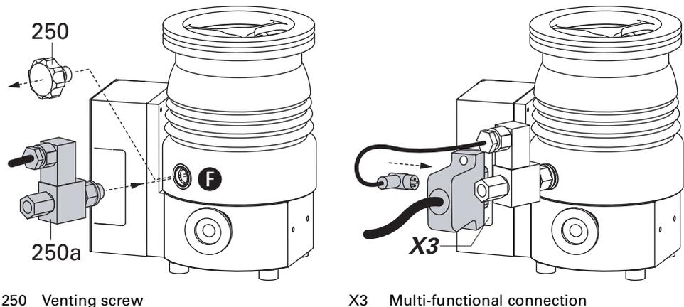
**Fig. 9: Connecting the venting valve**
