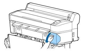
Hook a finger into the indentation on the top of the cartridge and pull it straight toward you.
