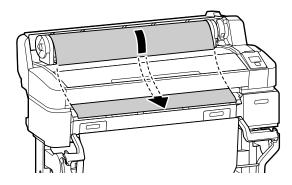
**11.** Rotate the roll paper adapters to push the paper straight through until the leading edge reaches the front of the printer.
