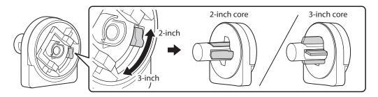
**5**. Release the tension lever on both adapters.
