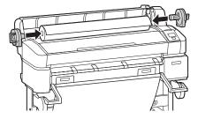
**7**. Push down the tension lever on both adapters to secure them.
