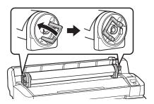
8. Slide the roll paper all the way to the right until it lines up with the adapter guides.
