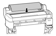
**4.** If necessary, adjust the roll media adapters to fit the core size of the roll paper.
