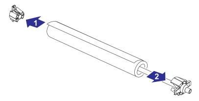
5 Remove the **new roll** from its wrapping, place it on the spindle, so that, as the media winds up from behind the roll, the media stop still on the spindle is on the right. Push the right media stop so that it is flush against the end of the roll (2 in the illustration below). Then insert the left media stop on the left end of the spindle.
