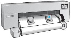
12 Align the edges of the media coming *out* of the printer with the same edges going *into* the printer, by pulling them taut with both hands and aligning them by eye. Make sure that the right-hand side of the media is aligned with the line of holes on the printer, and the roll. You may need to manually unroll a small amount of the media from its roll, to align the sheet satisfactorily.
