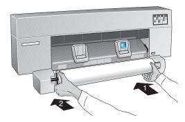
Make sure that each end of the spindle slots firmly into place with an audible "click".
