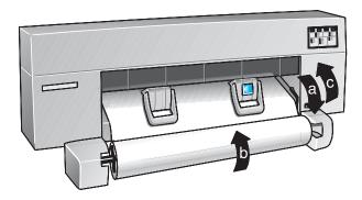
3 Remove the **old roll** by pulling firmly first on the left end of the spindle and then on the right. You may find that you have to push your thumbs against the cover of the roll-feed assembly while pulling the roll with your fingers to be able to release the spindle.
