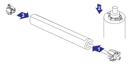
6 Put the loaded spindle back in the printer, pushing first the right side into place and then the left.
