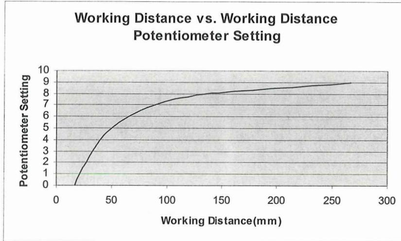
Figure 5. Showing the required setting for rear panel working distance correction potentiometer to compensate for changes in the raster size with working distance.
