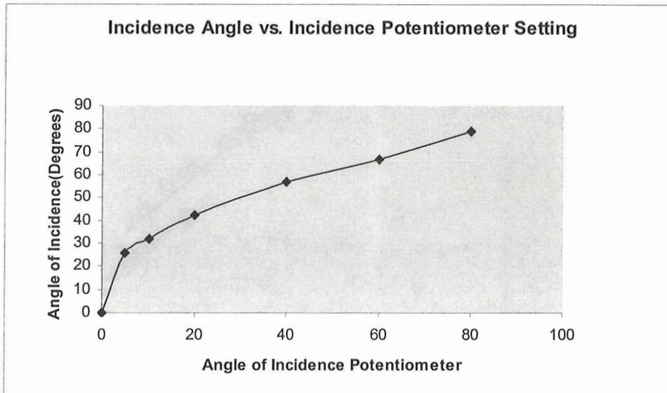
Figure 6. Showing the required setting for the rear panel Y- Incidence Angle Correction potentiometer in order to compensate for an oblique geometry.
