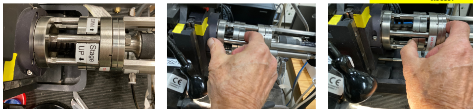
Figure 3. These pictures show the part that moves to raise or lower the stage. The left-hand picture shows the part that moves to control the stub is labeled. The right-hand figure shows how to push the movable piece, so the stage is fully up. The center picture shows pushing the piece, so the stage is fully down. The stage must be fully down to load and fully up to take data.
