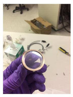
9. Reinstall the window holder in the chamber. This can be tricky, it may help to find something about 8-10" long with a flat surface on the end to assist in seating the window holder in the port.
