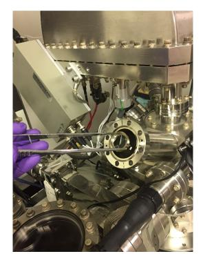
5. Place the window holder on a clean surface and remove the retaining ring from the holder.
