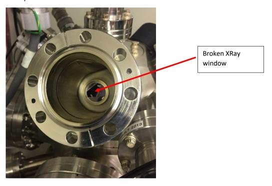
4. If the window is broken, use a pair of long tweezers to remove it from the vacuum chamber.
