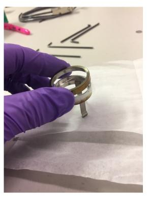
6. Remove the broken x ray window and all stray pieces of mylar.
