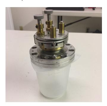
3. Look down the crystal port to examine the x ray window. If it is not broken, then reattach the crystal.
