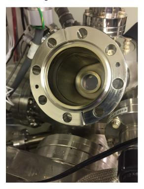
10. Reinstall the crystal. Be sure the crystal in facing towards the electron gun anode.
