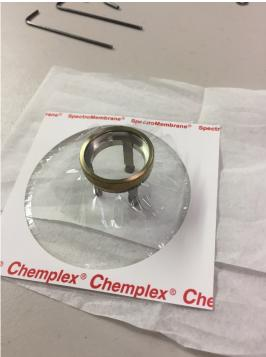
8. Remove excess film from the outside of the window holder.
