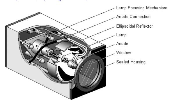
**WARNING:** Never look directly at an operating arc lamp; severe eye injury will result. Wear U.V. protective lenses, such as a welder's helmet, when working around operating arc lamps.
