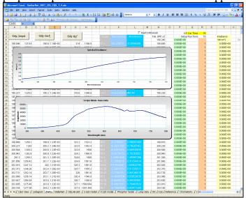
4. Go to the "Color View" tab and the "Reference" tab and verify that your results for x,y chromaticity and CCT match what was acquired in SpectraWiz. Please note that very small changes in measurement setup such as positioning of sphere head or receptor and software parameters may affect results. Additionally, scan to scan variance will also contribute to your measurement repeatability and accuracy. Increasing the amount of spectral averaging improves your results.
