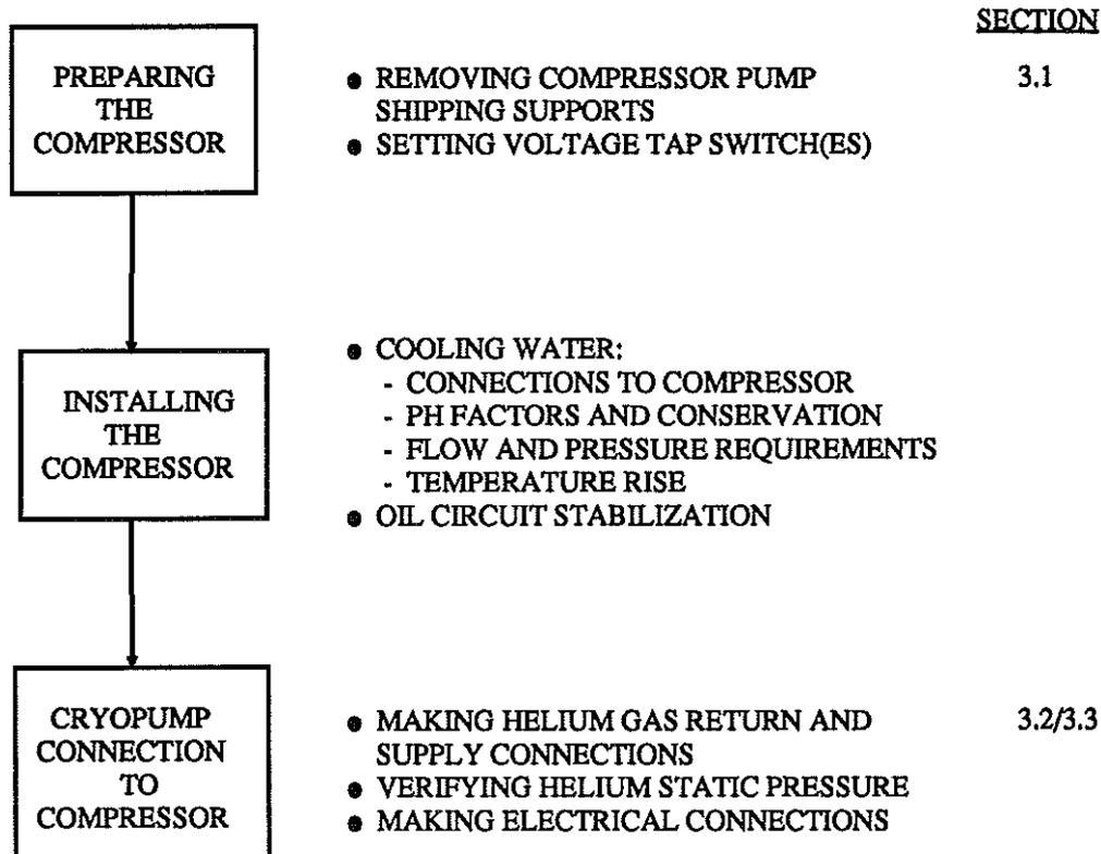
**Figure 3.1 Block diagram for 8500 Compressor Installation**
