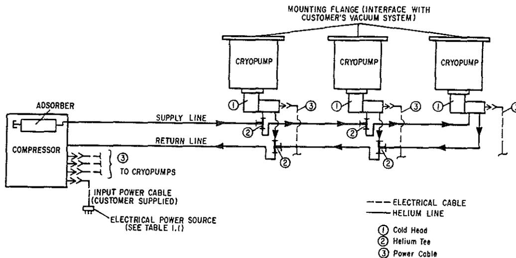
Figure E.1 Typical multiple cryopump installation with 8500 Compressor
