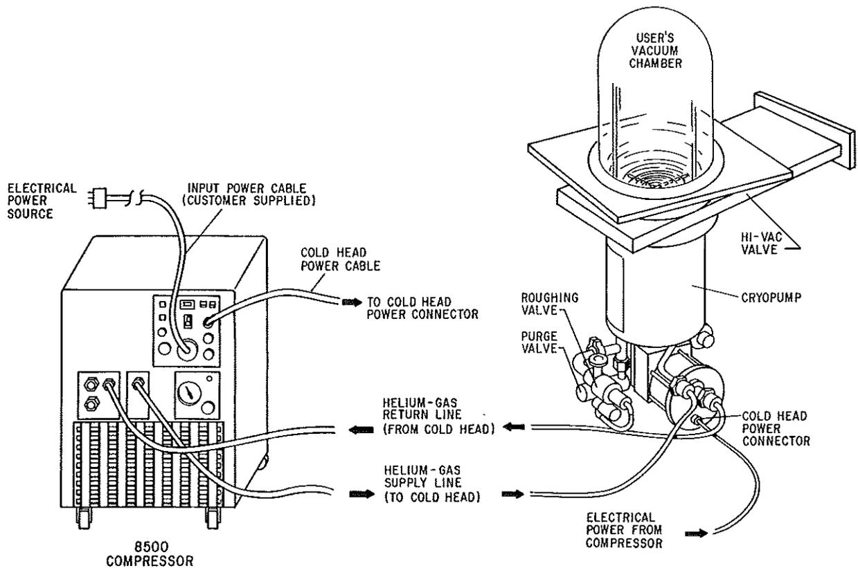
Figure 3.7 8500 Compressor installation
