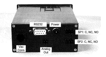
Take care in insuring that the wire connections are made fast, and the voltage and current does not exceed 250V or 7A. If you need to control a device that draws more power, consider another relay in between the Lesker output and the device to be controlled
