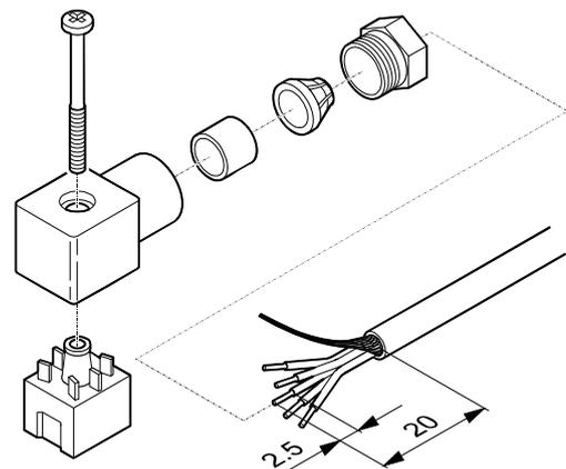
2 Solder the connection cable according to the diagram.
