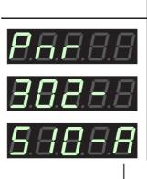
⇒ The two parts of the firmware number are displayed alternately.
