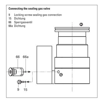
Please refer to Operating Instructions PM 800 229 BN for details on installing the sealing gas valve and adjusting the sealing gas flow.
