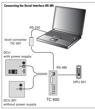
The serial interface is galvanically and safely separated from the maximum supply voltage from the TC 600.
