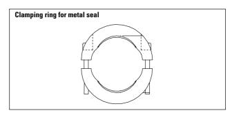
➡ The screws on the clamping ring need to be tightened with a tightening torque of 3.7 Nm.
