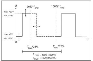
If no signal is present the pump accelerates up to its final rotation speed. A PWM adapter box for rotation speed setting operations for the turbopump is available as an option (please see "Accessories").
