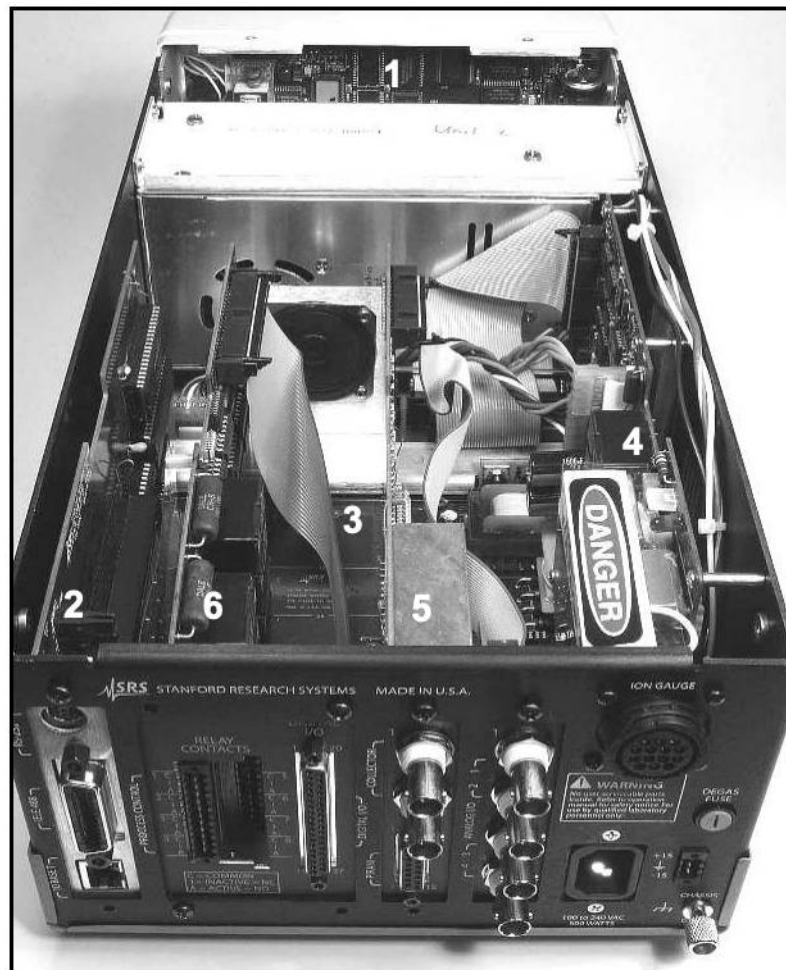
Figure N-1. Circuit board locations inside the IGC100 (rear view).
