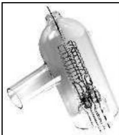
Figure E-1. Glass tubulated Bayard-Alpert ionization gauge, with glass side tube.
