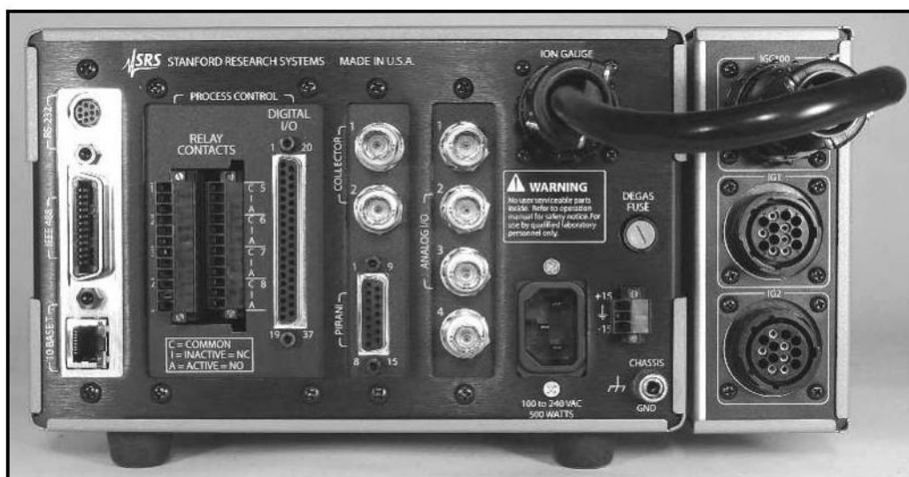
Figure L-5. Connect the IGC100 Ionization Gauge port to the OI00IG Box.
