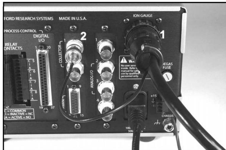
Figure 1-6. Single Ionization Gauge cable connection to the IGC100 controller.
