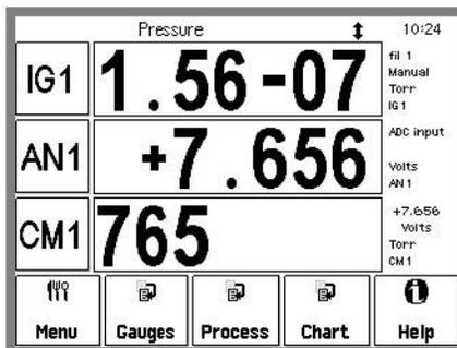
Figure 1-36. IGC100 displaying pressures from: IG1, AN1 and the CM pressure output signal at Analog I/O 1 port.
