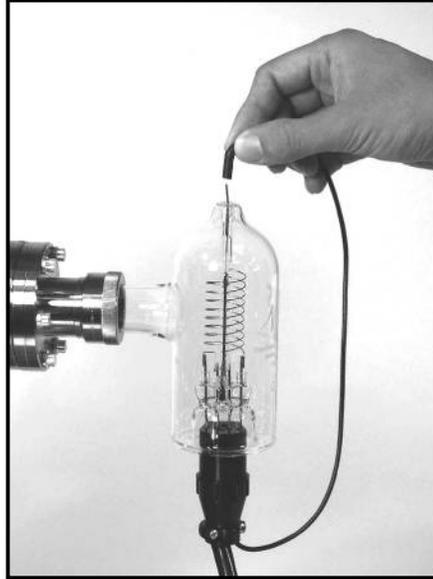
*Figure 1-10. Single pin connection to the collector electrode.*
