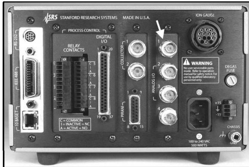
Figure 10-7. The four analog I/O ports.
