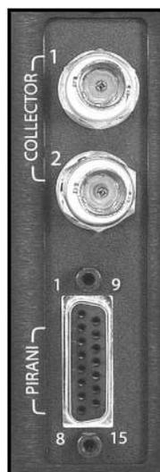
Figure 2-5. The Ion Gauge Collector BNC connectors.
