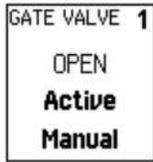
A Process Control Data Box displays the state (Active/Inactive), mode (Auto/Manual) and message for a single process control channel. Touch the Data Box to access the channel's rules and messages or to manually control its output.
