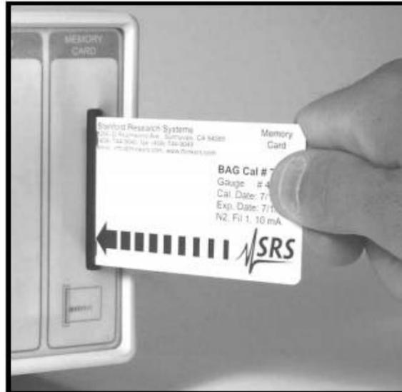
Figure 6-4. Insert the card into the controller.
