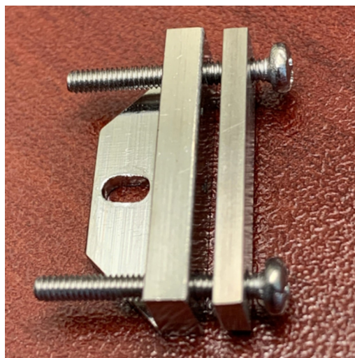
FIG. 12. Mini-vise can be used to mount samples for cross-sectional analysis. Image provided by Physical Electronics.
