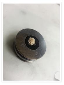
into the main XPS analysis chamber. Is the base pressure too high? Has the sample visibly changed appearance? If a problem is suspected, the RGA will give a fingerprint of the intro-chamber vacuum environment. If there is a huge background of water or organics-- do not introduce the sample into the XPS.
