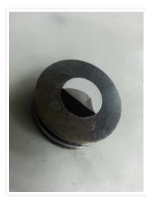
To remedy the complication of pressing samples into metal foils, as well as the corresponding spectral contamination, we have successfully used double-stick carbon tape used in SEM sample preparation. The mounting procedure is shown below:
