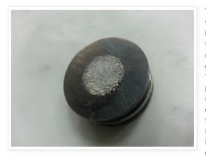
To get the stub ready for the XPS, tap the stub very hard on a rigid surface. Do this until there is no evidence of any powder coming off the surface. Tapping on a white weight paper can help. While it may seem that a good deal of powder has fallen off-that is acceptable. The XPS is a surface technique that looks at a few nano-meters of the sample surface. A fine dusting of material,
