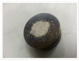
Step 3: A pile of powder will not make it into the the XPS safely. It should be noted that powders migrating through the XPS vacuum system is potentially very destructive to the instrument. Migrating powder can land on valve sealing surfaces causing them to leak and damage them so that they can never seal. Migrating powders can also destroy the turbo-
